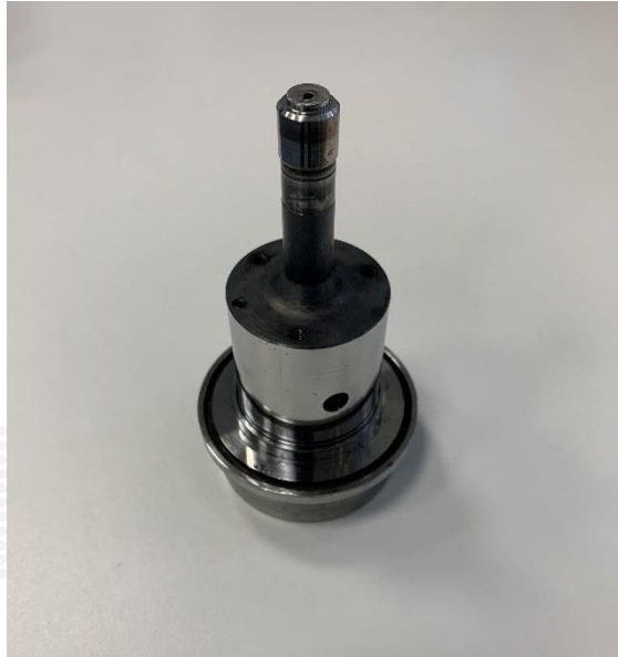
Figure 4: Drive gear shaft breakage
